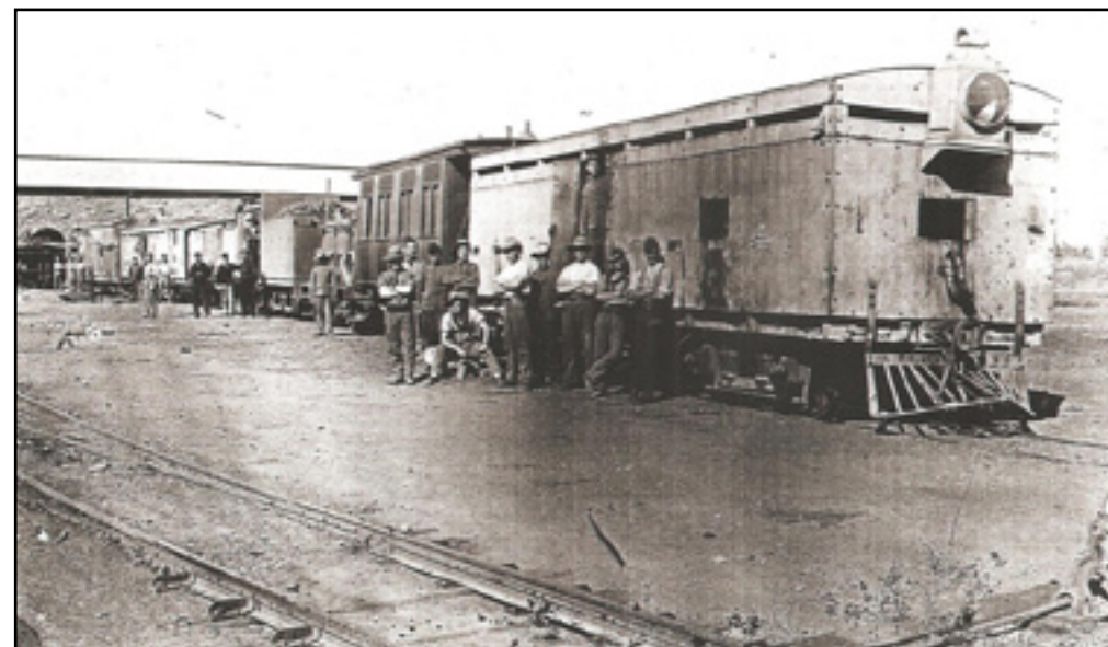
READY TO ROLL: Make up of a typical armoured train. Note that the locomotive is in the middle of the train, with armoured wagons on either side offering protection.
