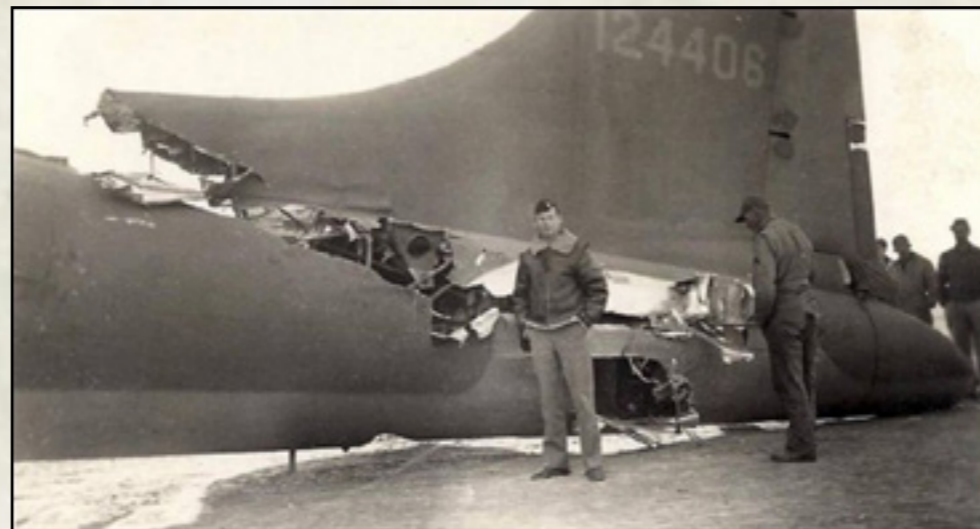
LUCKY TO BE ALIVE: A closer view of the extensive damage caused by the mid-air collision.
